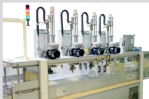
Enclosed polishing space with overhead polishing spindles
